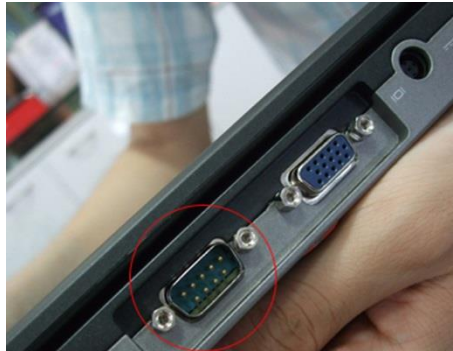
Built-in COM port (9-pin)
