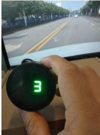
Figure 4. Press the selection button to adjust the volume.
