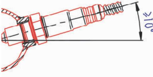
Recommended design of the mating thread in the exhaust pipe
