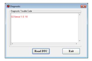
Click "Read DTC" button, GUI will read the active DTCs from ALM memory, example as in the above window. Refer to [chapter 3 DTC table] for all DTCs ALM supported.
