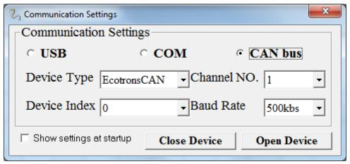
Step2: Click the button "connect" to connecting ALM to PC. It will points out "Connect successful!" in the lower left corner of the main window if all the options on Communication Settings window are correct and devices connecting errorless. But when you choose General CAN1 or EcotronsCAN, if the following prompt windows pop up:
