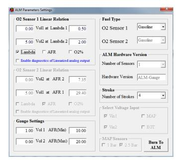
Lambda mode, ANOUT used to indicate changes in lambda, the default setting:
