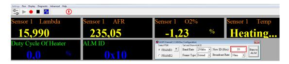
Example 3: change FRAME1 of channel 1 baud rate to 500kbs.
