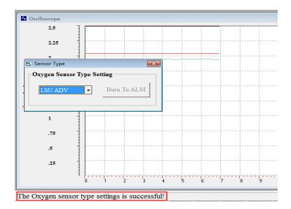
3. After you have changed the sensor type successfully, click "Disconnect" and power off the ALM, change the LSU ADV sensor replacing the former LSU 4.9.
