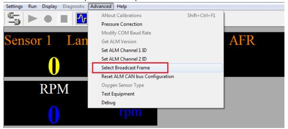
Step8: Opt for one or two Frame and click "OK". Select two Frame the image below. When click "OK", the reminder "Select the number of CAN channels!" will appear in the lower left corner of the main window.
