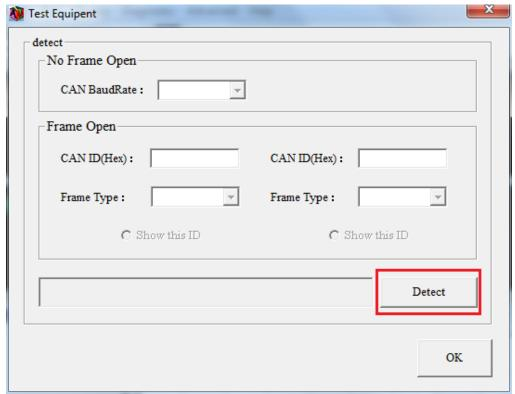
Step5: If the prompt window shows "Can not detect device", you should check for the cause of the error. There are several reasons lead to this situation, maybe the connection between the CAN device and ALM is reversed or the ALM is not power on. Please power on the ALM and correct wiring first.
