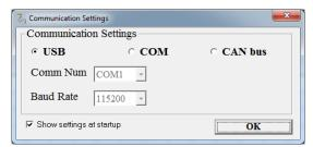
CAN bus method is used to communicate with ALM with CAN bus. If you are using CAN communication, select the USB-CAN Device Type. ALM GUI currently supports the Ecotrons and Kvaser USB-CAN device; the future will support more manufacturers. Ecotrons USB-CAN-Z device is compatible with ZLG, if you are using Ecotrons USB-CAN-Z, device type selection ZLG.
