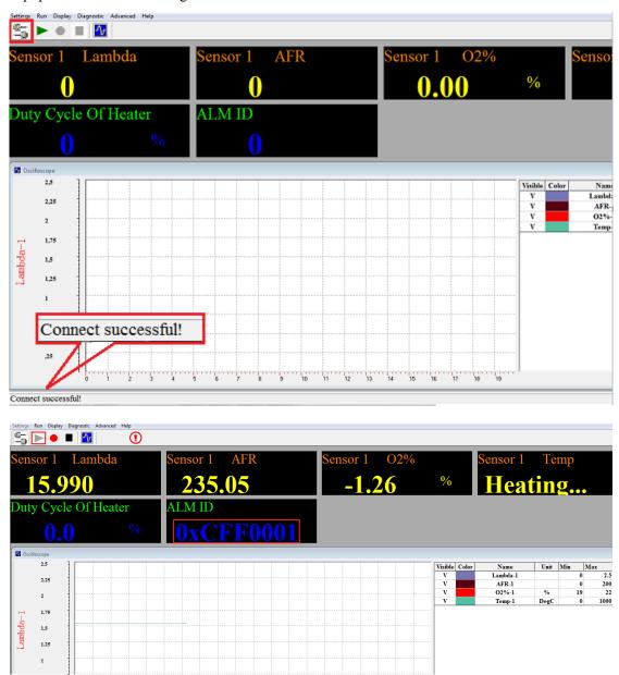
Step11: If there is only one ID in the "Test Equipment" window, the ID will be as Frame2 to display. When the screen displays FRAME2 (FRAME61454) data, because ALM only supports O2% of FRAME61454, so in the ALM GUI, lambda, temperature, etc. default display is 0.
